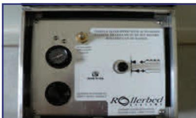
System air is fed via nylon air lines, featuring easy push-in connectors, from the auxiliary air tanks to the stainless steel control box containing a pressure regulating valve and air control valves. Typical plumbing is designed for ease of operation; one push-pull valve will raise and lower the entire system. Pneumatic plumbing layouts can also be designed for custom applications.
