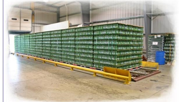
The conveyor can be installed on top of a framework or fitted flush with the floor dependent on the relative heights of the trailer and internal facility floor. The chain driving unit is normally located at the front and below the dock, but can be side or pit mounted at the rear.
